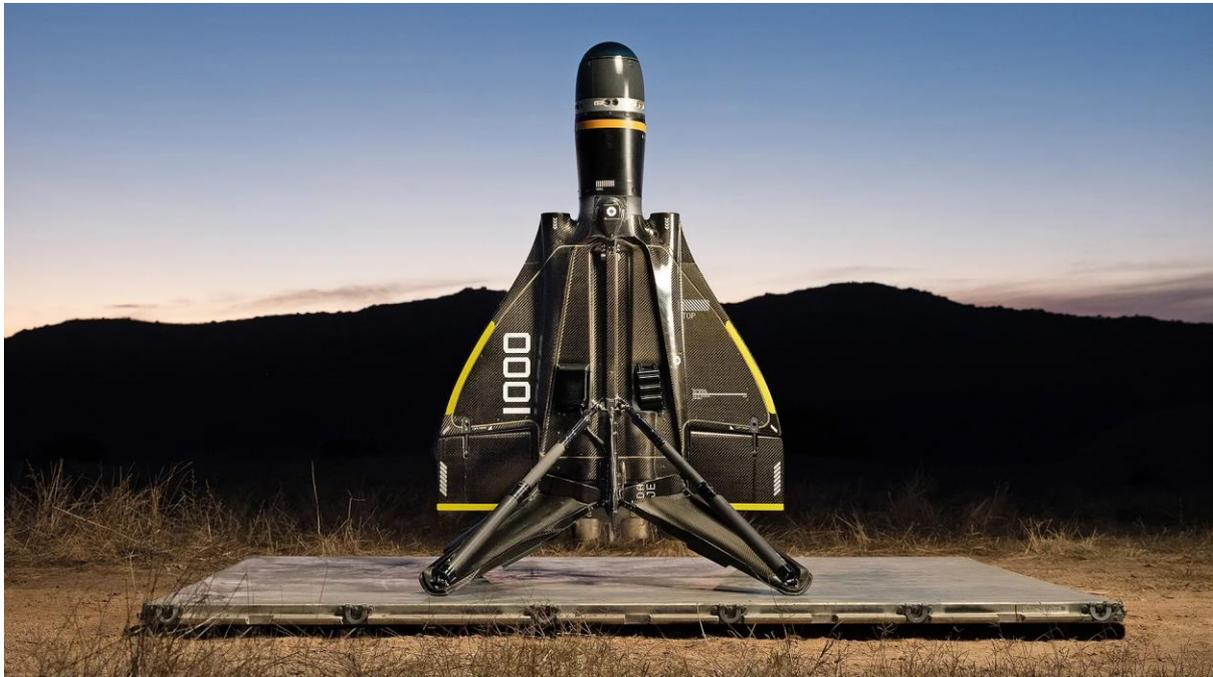
Image 1: Roadrunner is a twin-jet-powered drone
